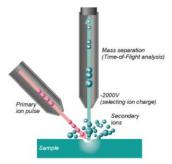
TOF-SIMS (Time-of-flight secondary-ion-massspectroscopy) Instrument for mapping the chemical composition of a material within a few nano-meters (Niels B. Larsen, Risø) In this report, we use the concept nanotechnology for technologies which exploit the new possibilities for structuring materials at the sub-micrometer scale – either chemically or physically. At this scale, new properties can be achieved which cannot be created using conventional technology.
