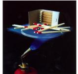
Matches On Aerogel Over A Flame Another photo illustrating the excellent insulating properties of aerogel. The matches on top of the aerogel are protected from the flame underneath.
