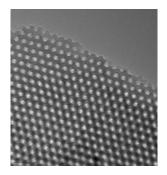
Electron microscopy picture of a nanopourous polymer material based on a block copolymer. (Sokol Ndoni, Risø)
