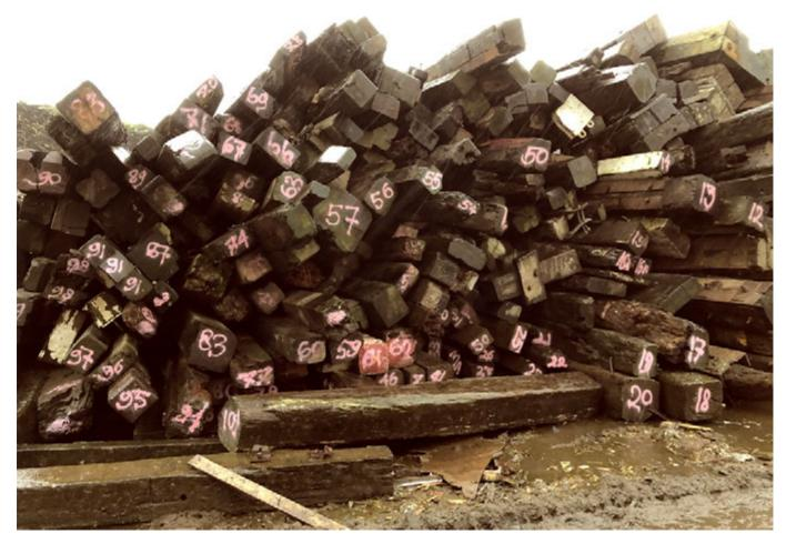
Wooden fender poles were specifically identified and measured so that the linear programming model could optimise their shape and layout on the final structure (Source: Boris Zeisser)
