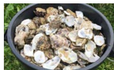
Shell material For floor sub-base
