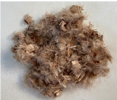
Bull-rush fibre from Hedeskov that will be added to the clay plaster topcoats
