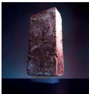
A 2.5 kg brick is supported on top of a piece of aerogel weighing only 2.38 grams (NASA)
